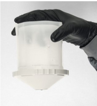
Cup A: The vented hard cup system dispensed all fluid in the cup, but produced a stop and go "glugging" restriction that creates an inconsistent paint flow.
