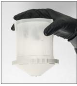
**Competitor A:** The vented hard cup system dispensed all fluid in the cup but produced a stop and go "glugging" restriction, creating inconsistent paint flow.
