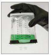
**Competitor B:** The liner system created a highly restricted condition in the liner, showing that it would starve the spray gun. **The final 8 oz. of fluid in the cup would not flow out of the cup.**
